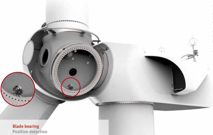
In addition to rotational speed and position acquisition on the pitch motor, it is possible to determine the rotor blade position almost free of play using a rotational speed acquisition at the root of the blade. For this purpose an absolute rotary encoder with integrated bearings is fitted with a flexible flange; this encoder engages directly with the teeth on the blade bearing.
