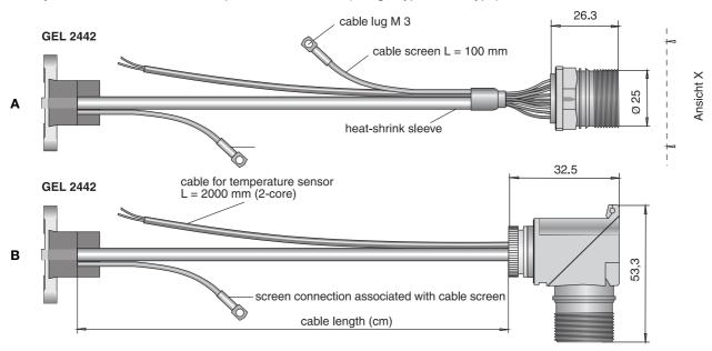
Important: Fit the cable screening as coaxially to the earth cable as possible. When fitting the cable screening onto an earth cable, the earth cable should be run as short as possible.
