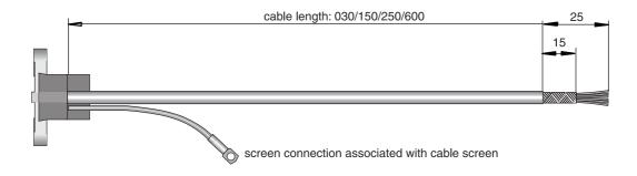
Important: Fit the cable screening as coaxially to the earth cable as possible. When fitting the cable screening onto an earth cable, the earth cable should be run as short as possible.
