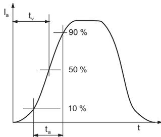
Rise time  $t_a$  and delay time  $t_v$  after a erratic change in speed
