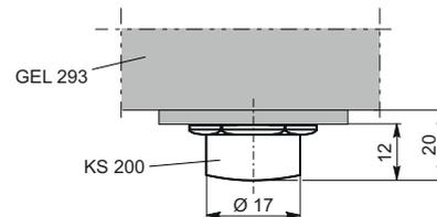
The position of the condensed water outlet must be specified when ordering.
