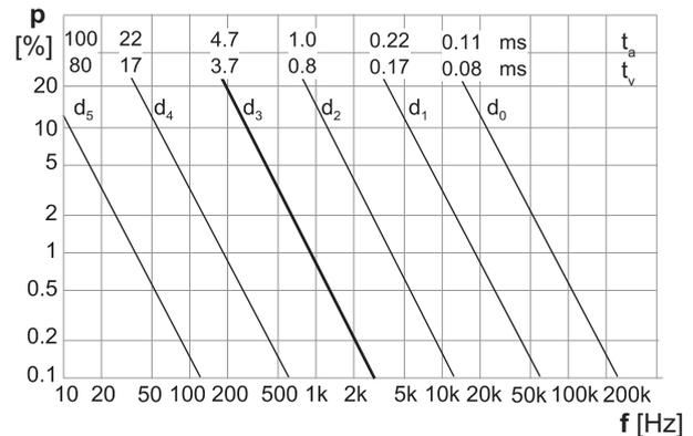
Harmonic content of the output current as a function of the pulse frequency ( $f$ ) and the selectable attenuation ( $d_n$ )
