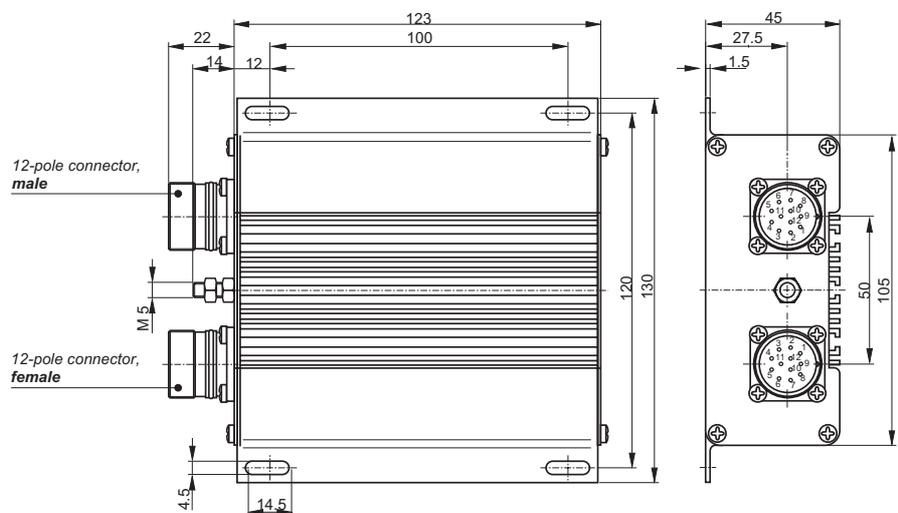
Make sure that the cable screening has large-surface contact with the connector housing.
