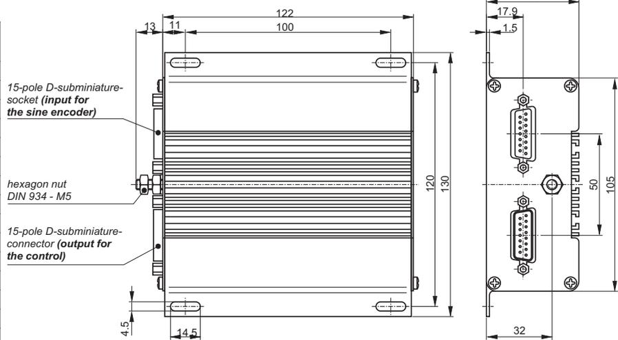
Make sure that the cable screening has large-surface contact with the connector housing.
