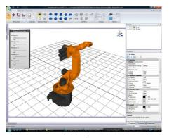
scenarios quickly and easily. GraphWorX64 supports the import of other 3<sup>rd</sup> party 3D models from Autodesk (.dwg, .dxf) and other standard file formats like .3ds, .dae (COLLADA) and .obj. Customers with existing models can import and use them for HMI displays. Users can also combine EarthWorX with their 3D models by using the 3D Terrain feature. By adding a Terrain
