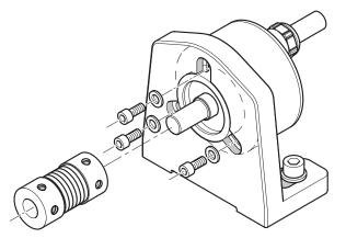
• Mounting using a clamping device
