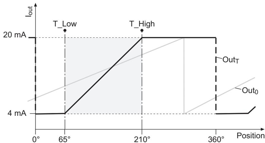
$Out_0, Out_T$  Output signal graph before (index 0) or after (index T) the adaptation via the teach-in signals; the desired working range is shaded in grey, the degree specification on the x-axis is selected arbitrarily
