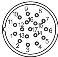
Connector socket (pins, connection side view)
