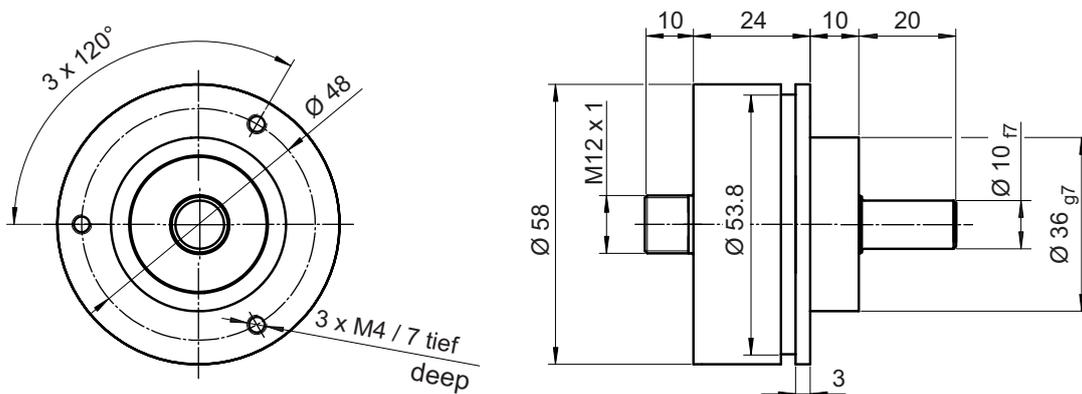
**Semi hollow shaft (only GEL 2352 and GEL 2035)**
