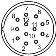
Connector socket (pins, connection side view)
