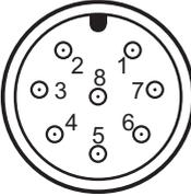
Connector socket (pins, connection side view)
