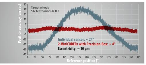
Achieve positioning accuracies in the range of a few arcseconds in your application! The Precision-Box processes analog signals from two MiniCODERs mounted opposite each other. The eccentricity error is minimized dynamically even at high speeds far in excess of 50,000 r.p.m.
