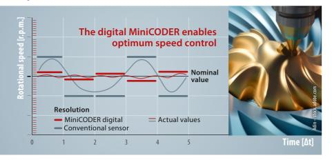
The 26 bit resolution is available up to a maximum speed of 100,000 r.p.m. Improved surface quality can be achieved by increasing control accuracy. The integrated signal conversion also allows precise positioning in the scope of a few arcseconds.
