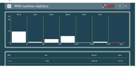
Our MiniCODERs offer the possibility of integrated operating state data acquisition. Operating conditions such as minimum and maximum temperatures and speed ranges are recorded during runtime. In the event of a service or warranty claim, for example, it can be used to check whether a motor has been operated above permissible speed.
