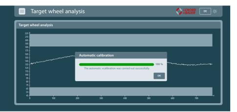
The mobile service unit SensorDEVICE M can be used to calibrate the MiniCODERs while they are installed. During the adjustment process, the signal quality of the sensor is improved, which allows higher position accuracy to be achieved.
