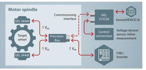
In order to achieve a positional accuracy in the range of a few arcseconds, the Precision system can be parameterized and the signal quality optimized with the SensorDEVICE M mobile service unit after installation. The SensorDEVICE UI user interface provides the user with an intuitive commissioning wizard that guides the user step-by-step through the setup of the Precision system. In this way, errors during commissioning can be avoided and the assembly time can be shortened.
