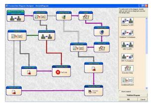
The key concept of BridgeWorX is the transaction. A transaction is a set of data-transfer tasks (operations), defined by the user, to be executed in a user-configured order. A transaction represents a user-configured flowchart of data operations and data transfers, prioritized by the user, with optional precedence constraints (e.g., do step 2 only if step 1 succeeds) and completion actions.
